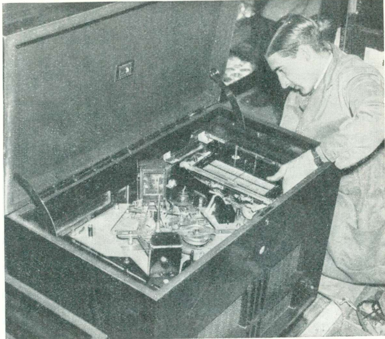
PUTTING THE FINISHING TOUCHES TO A BIG SET An H.M.V. engineer fixing in the radio chassis in one of the nine-valve automatic record changing radiograms. It will be seen that the "motor board" carries no weight at all. A smart-looking outfit, you will agree!
