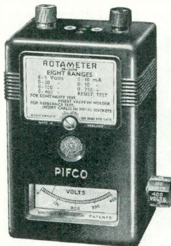
A reasonably priced multi-range test meter, the moving-coil Rotameter is ideal for amateur requirements
