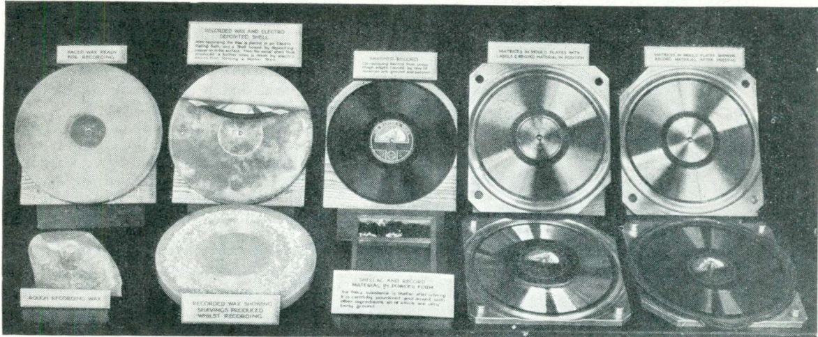
Fig. 1. —An interesting photograph showing the complete process from the rough wax, on the left, to the finished record in the centre. Readers should be able to read most of the wording on the cards with an ordinary magnifying glass
